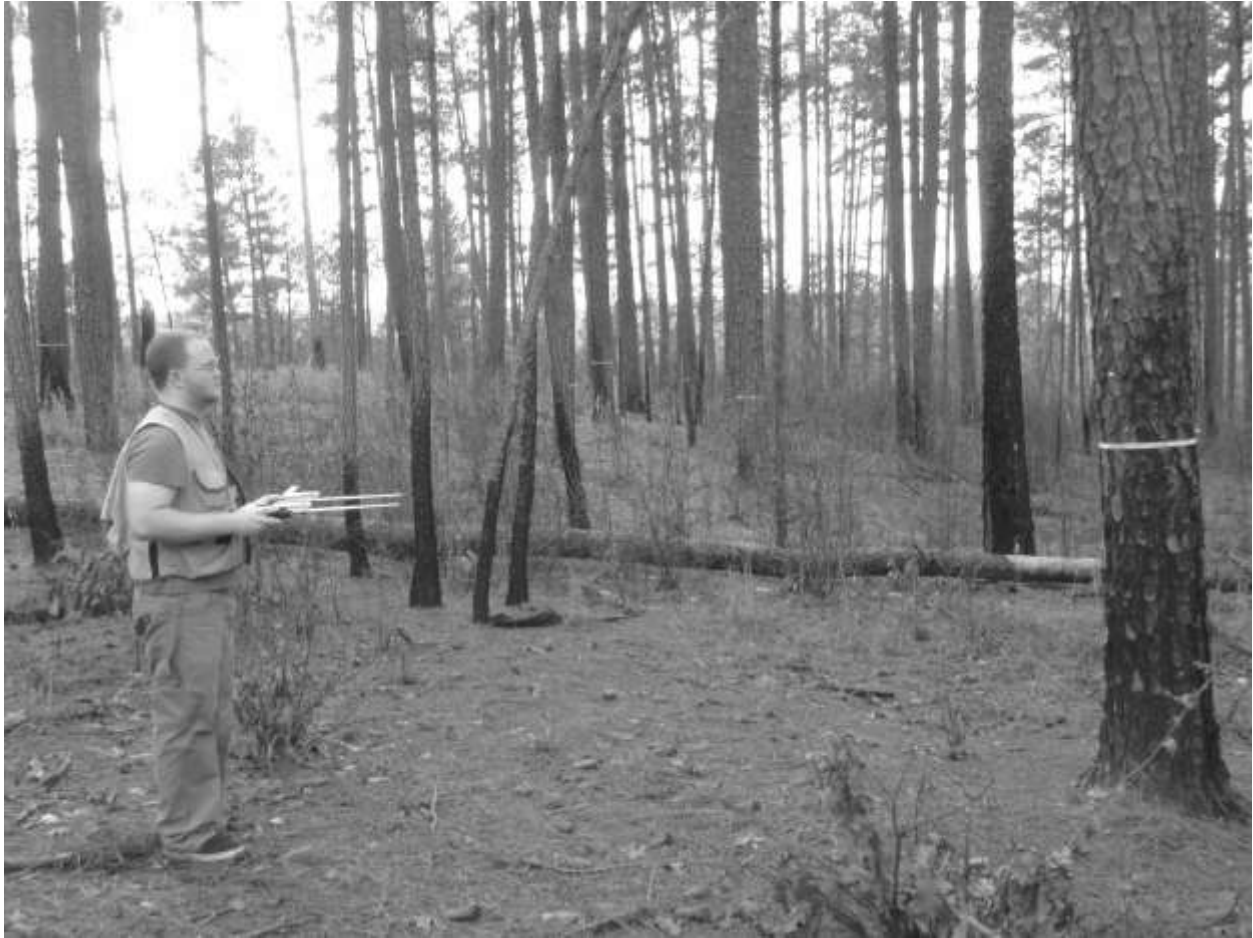
Figure 2.3. Diameter measurements conducted at a distance with the laser caliper dendrometer.
