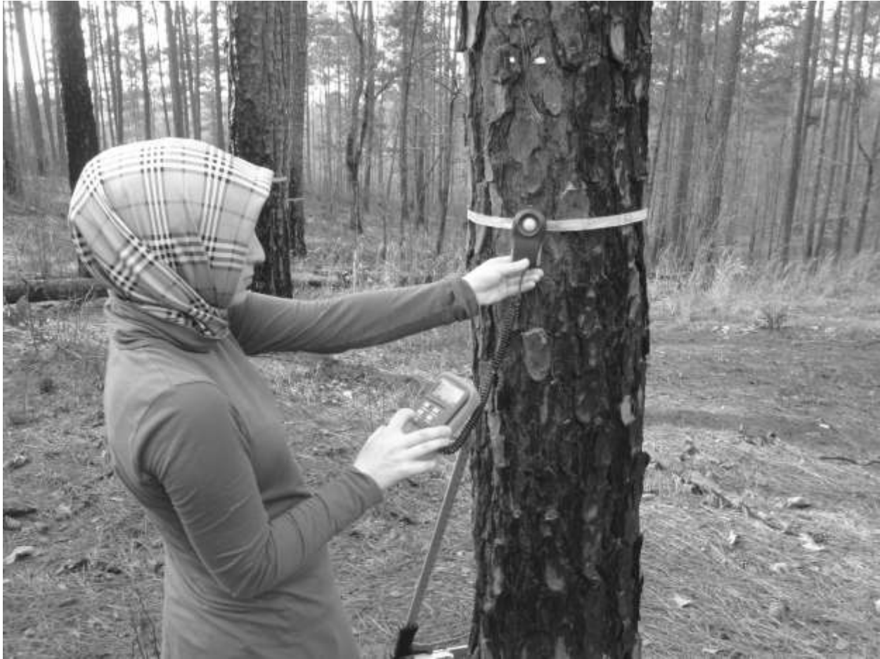
Figure 2.5. Light conditions being measured using the Mastech LX1330B light meter.
